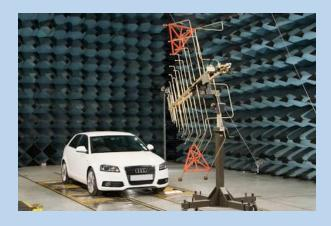
ARAI is setting up vehicles EMC facility suitable for testing of passenger cars and light commercial vehicles at ARAI, HTC Chakan. This facility will support industry for EMC compliance of conventional as well as Electric and Hybrid vehicles.
